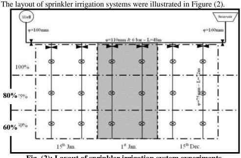
Fig. (2): Layout of sprinkler irrigation system experiments.
